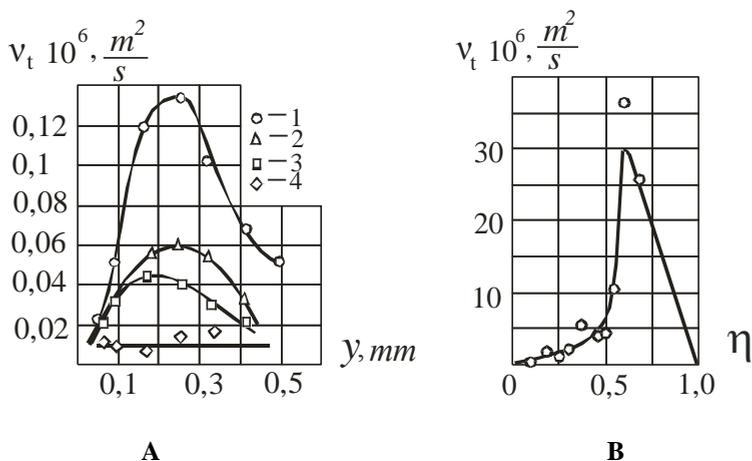
**Figure 1.** The dependence of turbulent viscosity on the film thickness of water ( $t = 20^\circ C$ ).
