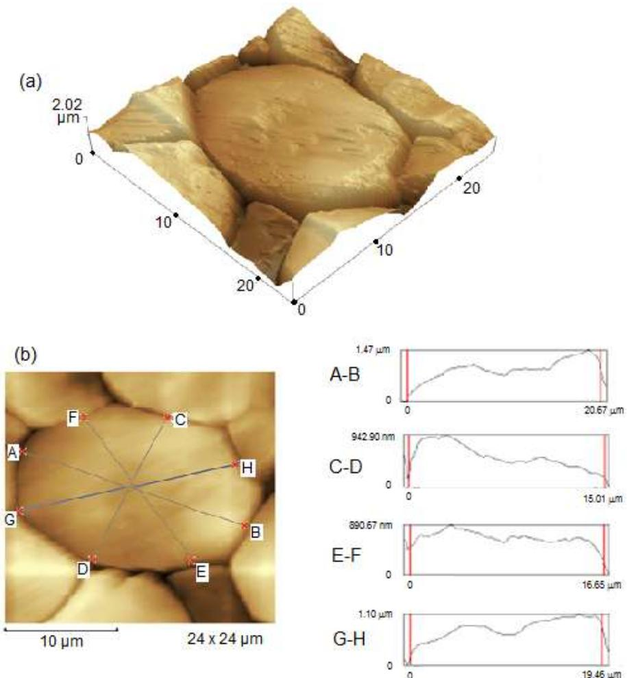
**Figure 3.** NC-AFM, 3D (a) and 2D (b) topographic micro-images of untreated “pinhão” starch granules (scan size 24 x 24  $\mu\text{m}$ ), height difference 2.02  $\mu\text{m}$ , and the cross section
