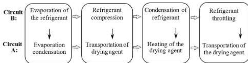
**Figure 2. Synchronization of processes in the circuits A and B from Figure 1**
