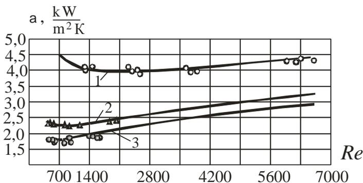
**Figure 4.** Dependence  $\alpha = f(\operatorname{Re})$  for water and sugar solutions in a pipe with a diameter of 20 mm, length  $L = 1,5$  m,  $t = 100$  °C.
