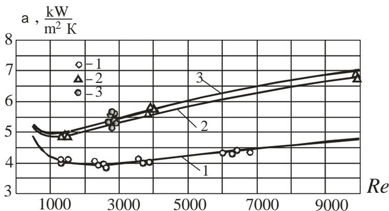
**Figure 5. Dependence  $\alpha = f(\text{Re})$  for pipes of different diameters.**
