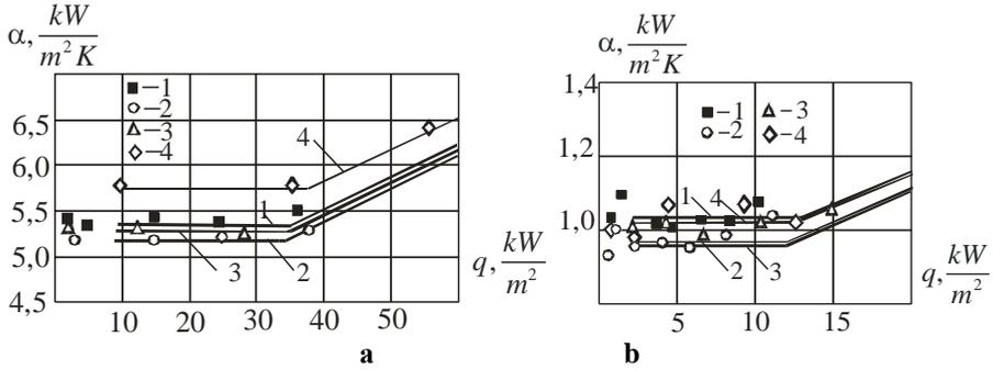
**Figure 12. Dependence  $\alpha = f(q)$  during the movement of steam with speed  $u_2 = 25 \frac{m}{s}$ .**
