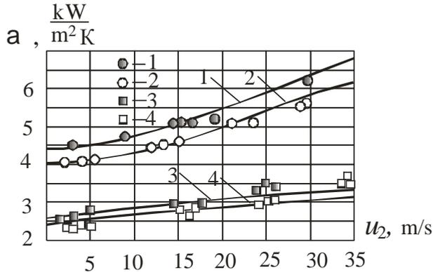
Figure 9. Dependence  $\alpha = f(u_2)$  for water and sugar solutions for the pipe,  $d = 20 \text{ mm}$ .
