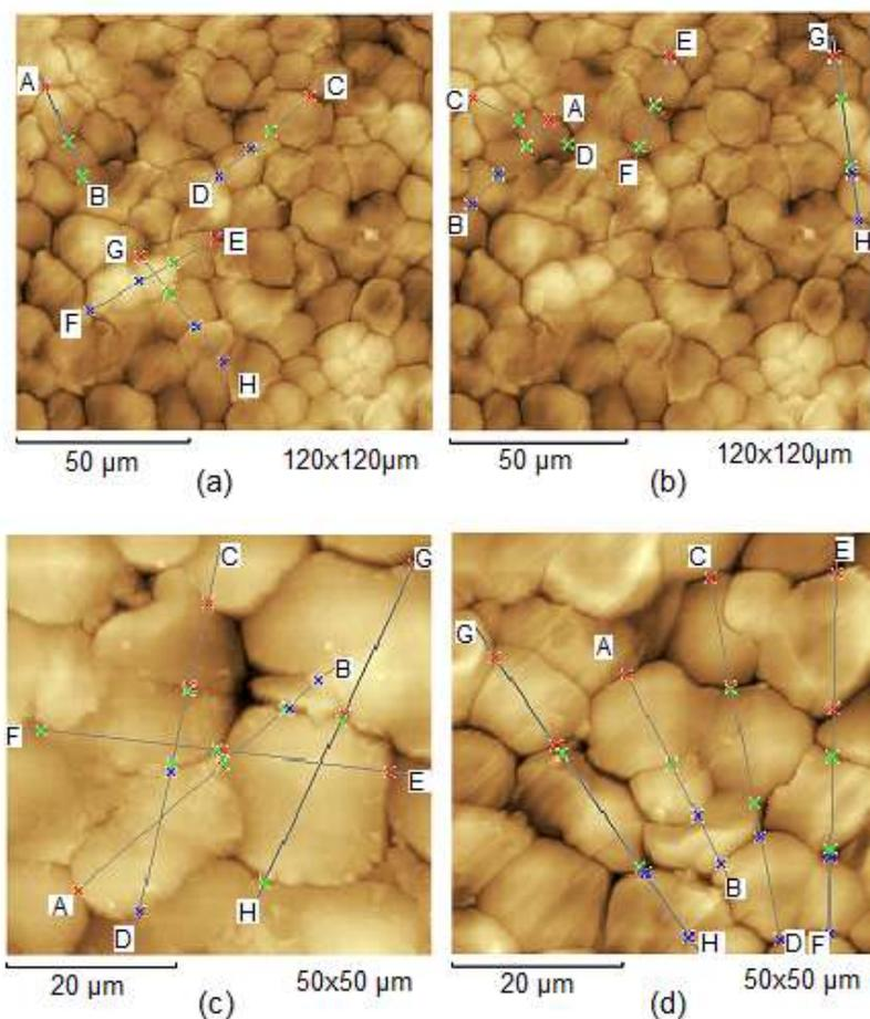
**Figure 4:** NC-AFM, 2D micro-image of untreated “pinhão” starch
