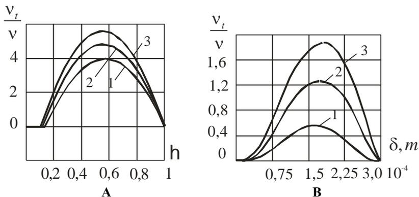
**Figure 2. Distribution of turbulent viscosity in the cross section of the film by relations (1) and (2).**
