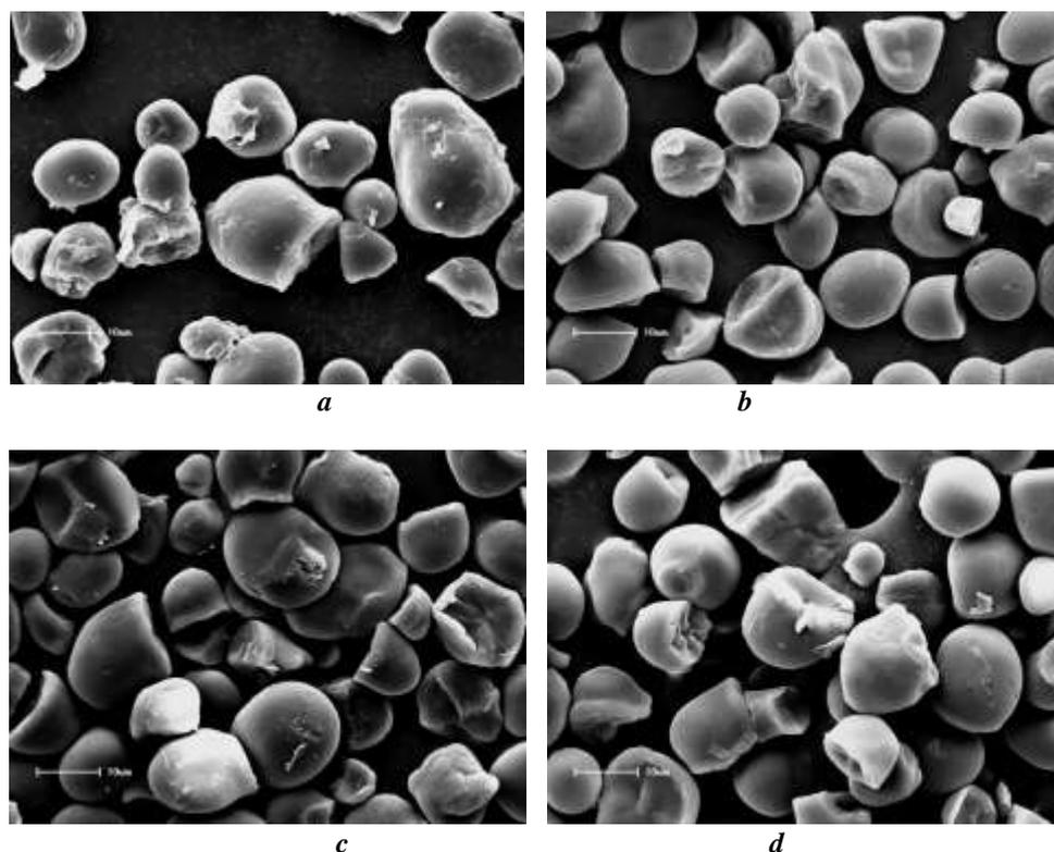
**Figure 2. Scanning electron microscopy (SEM) of “pinhão” starch granules (a) untreated; (b), (c), and (d), treated by HMT (magnification 1200 X, bar 10 µm)**
