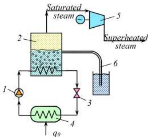
Figure 4. Heat pump circuit
