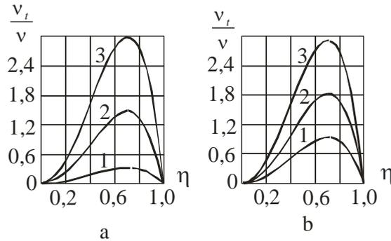
**Figure 8.** Dependence  $\frac{v_t}{\nu} = f(\eta)$  on the ratio (17) for water at  $t = 100^\circ \text{C}$ ,  $d = 0,02 \text{ m}$ .
