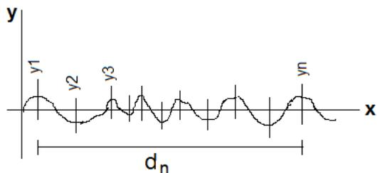
**Figure 1. Measurements of average roughness ( $r_a$ )**
