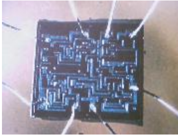
A medium-scale integrated circuit die, with bond wires attached.
