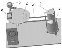
reverse disk which receives movement from the drive through pass transmission. A disk material - a steel, a surface roughness - 0.8. Rate of slippage in a place of contact to bread varies from 0.5 to 7.5 m/s. On a disk surface in a header place a piece of bread in the size 4x4x2 mm. At disk rotation between bread and a disk there is a friction force which is registered a dynamometer. The specific load on a friction surface varies with weights.
