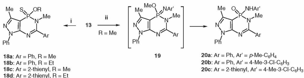
**Scheme 6** Reagents and conditions: (i) S, py, r.t., 12 h; (ii) ArN<sub>3</sub>, py, r.t., 5 min; (iii) ROH, py, r.t., 10 min
