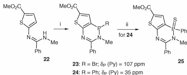
**Scheme 8** Reagents and conditions: (i) for **23**:  $\text{PBr}_3$ , py, r.t., 3 h; for **24**:  $\text{PhPBr}_2$ , py, r.t., 3 h; (ii) S, py, r.t., 1 h.
