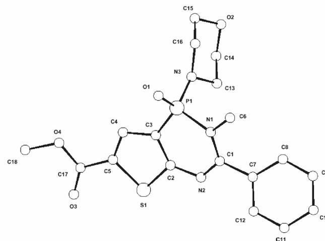
**Figure 2** Structure of cyclic phosphine oxide **27**. Selected bond lengths (Å) and angles (°): P(1)–O(1) 1.471(1), P(1)–N(1) 1.717(1), P(1)–N(3) 1.645(2), P(1)–C(3) 1.750(2), S(1)–C(2) 1.732(2), S(1)–C(5) 1.733(2), N(1)–C(1) 1.374(2), N(2)–C(1) 1.304(2), N(2)–C(2) 1.360(2), C(2)–C(3) 1.381(2), C(3)–C(4) 1.421(2), C(4)–C(5) 1.357(3); N(1)–P(1)–C(3) 99.5(1), C(2)–S(1)–C(5) 91.2(1), P(1)–N(1)–C(1) 125.6(1), C(1)–N(2)–C(2) 119.0(1).
