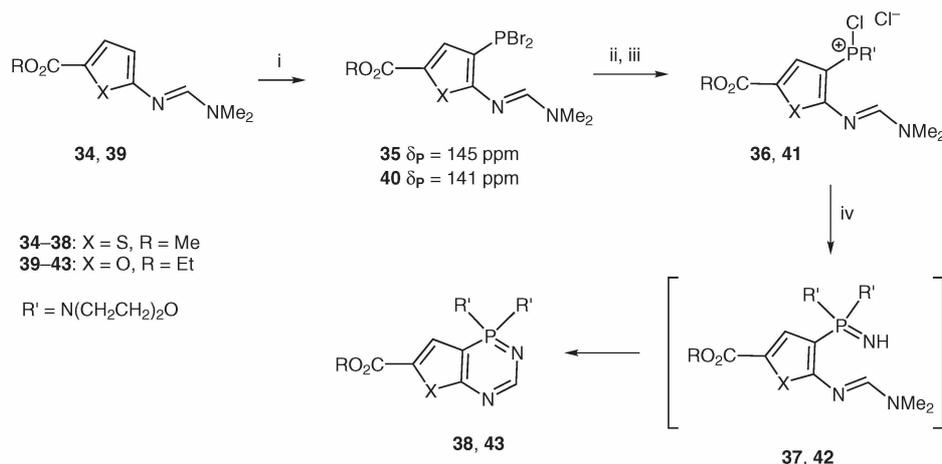
**Scheme 11** Reagents and conditions: (i) PBr<sub>3</sub>, py, r.t., 12 h; (ii) amine, Et<sub>3</sub>N, py, 1 h; (iii) C<sub>2</sub>Cl<sub>6</sub>, PhH; (iv) NH<sub>3</sub>, CH<sub>2</sub>Cl<sub>2</sub>, 24 h.
