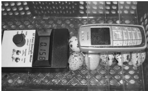
FIGURE 2 Irradiation of quail embryos in ovo (exposed group) to MWs of commercial GSM 900 MHz cell phone in a plastic incubation tray within the incubator.
