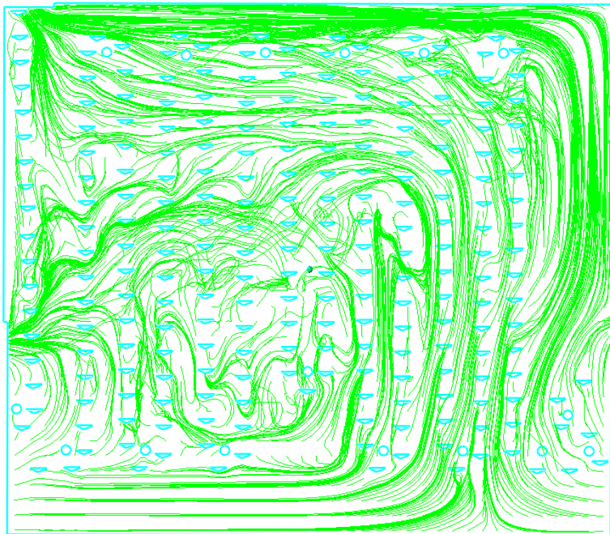
Fig. 4. The trajectories of the air in the proofer RSV.
