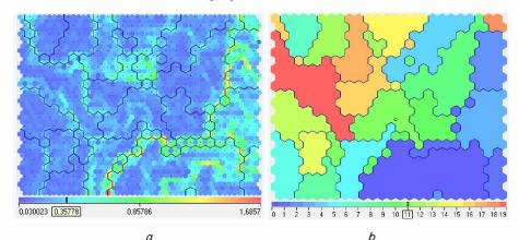
Fig. 5. Result of clustering (number of epochs -200; size of the output grid of neurons  $-25 \times 22$ ; automatic determination of the number of clusters): a - matrix of distances; b - map of splitting into clusters
