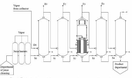
Fig. 1. Typical scheme of five-case evaporation station of sugar factory
