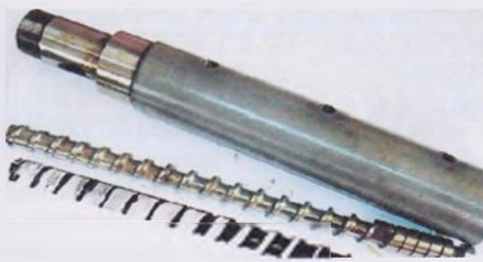
Fig. 2. Physical appearance of the screw extracted from an extruder body (light color highlights the melt solidified in the screw channel)
