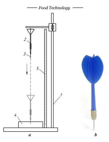
**Figure 1. Experimental device: a – experimental device; b – penetrometer;** 1 – tripod; 2 – dart; 3 – needle; 4 – products; 5 – straightedge.
