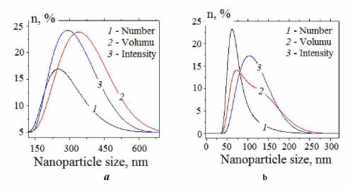
Figure 2. Distribution of silver nanoparticles in solution before (a) and after (b) ultrasonic treatment.
