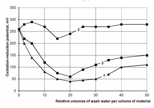
Figure 6. Water oxidation—reduction potential of the prepared water using activated shungite, activated and treated by nanosilver shungite, activated, steam and nanosilver treated shungite.
