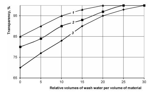
Figure 4. The consumption of flushing water at the stage of shungite preparation: 1 – shungite sample activated, steam treated and modified by nanosilver;
