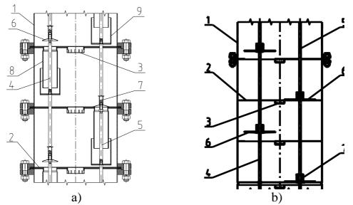
Figure 1. Fragments of the studied RC with movable valves: with hydraulic shutters (a) and without hydraulic shutters (b): 1 – body; 2 – plates; 3 – contact devices; 4, 5 – rods; 6 – valves; 7 – springs; 8 – pouring pipes; 9 – glasses.
