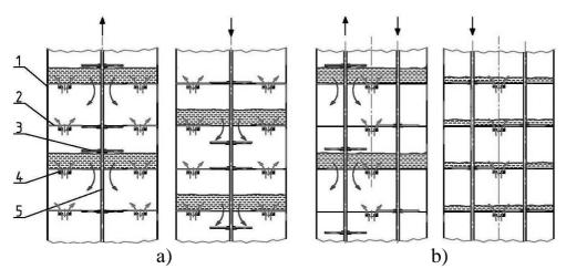
Figure 2. One-stage and two-stage methods of liquid pouring on the plates of the cyclic action RC:
