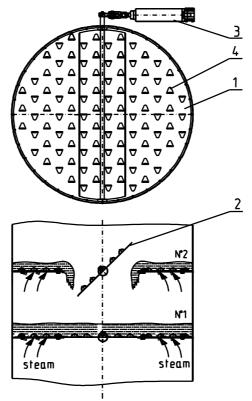
Figure 4. Flaky plate of cyclic action with coaxial placement of flakes and variable free cross-section 1 – plate fabric; 2 – moving section; 3 – drive mechanism (pneumatic cylinder); 4 – flakes.
