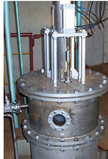
Figure 2. Fragment of a prototype LC with movable valves:
