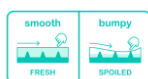
Fig. 2. Tactile freshness indicator by Mimica: smooth surface (fresh) vs bumpy surface (spoiled)
