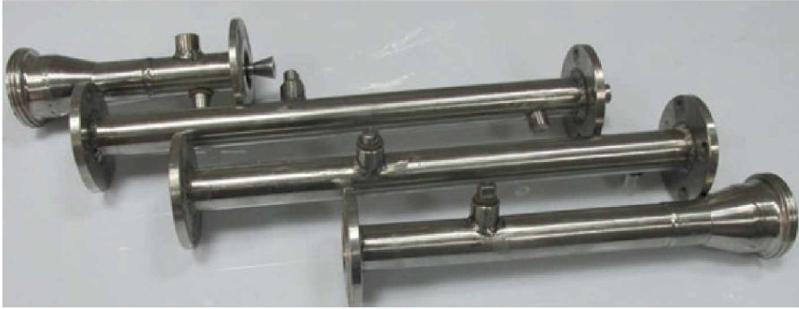
Fig. 1. Experimental samples of cavitation devices
