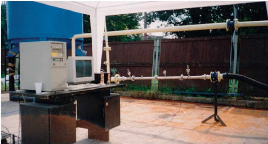
Fig. 2. Experimental stand for hydrodynamic cavitation
