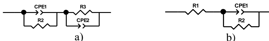
Fig. 3.2. Equivalent schemes of suspensions based on aerosol 300-NED of black radish (a) and white cabbage (b).
