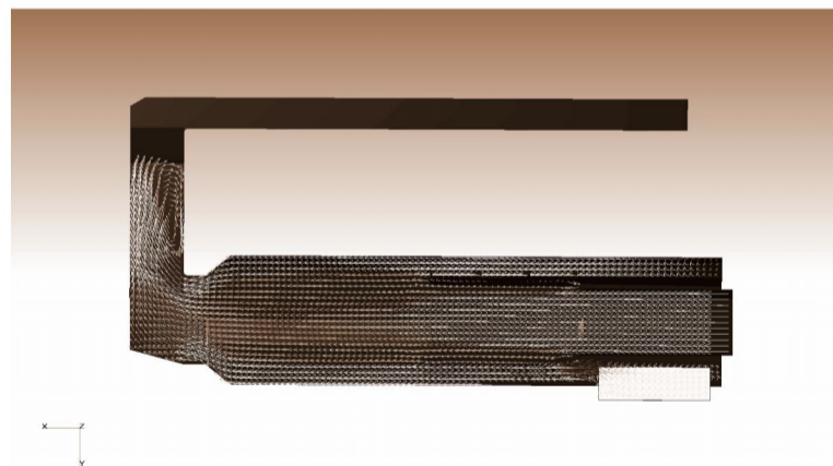
Figure 3. Velocity vectors of the gas in the furnace furnace
