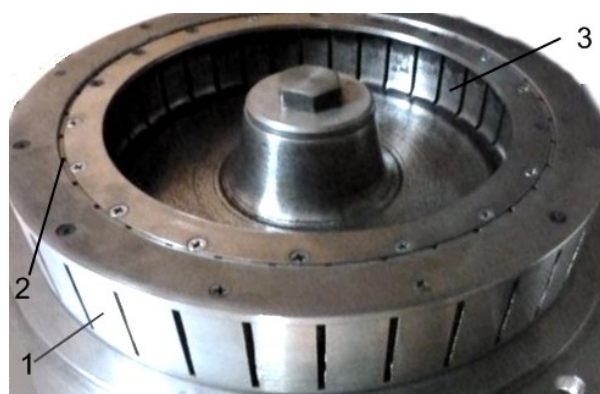
Figure 1. The working chamber of the rotary pulsed apparatus: 1 – external rotor; 2 – stator; 3 – internal rotor
