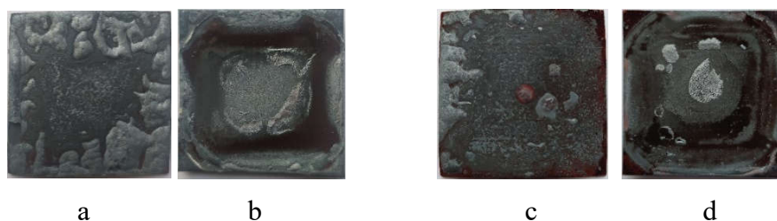
Fig. 1. The influence of salty (a, b) and desalted (c, d) coal on metal surfaces
