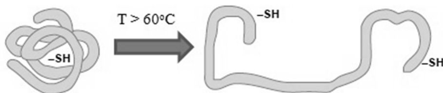
Figure 3. Schematic representation of \beta -lactoglobulin denaturation: breakage of its tertiary structure and exposure of thiol groups
