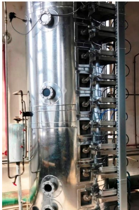
Figure 2. Experimental column with controlled mass exchange cycles between liquid and vapour
