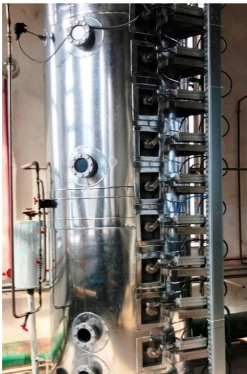
**Figure 1. General view of a impurity concentration column**
