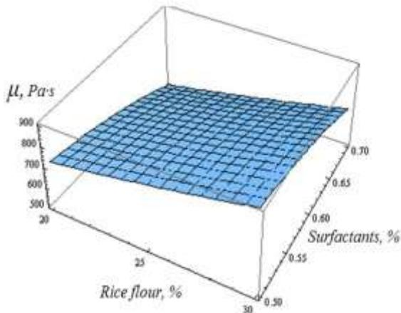
**Fig. 2. Response surface of dosing rice flour and surfactant on viscosity of dough for special purpose fondants**
