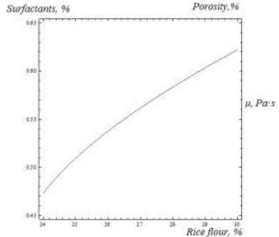
**Fig. 3. The line of viscosity of fondant dough depending on rice flour and surfactant dosage**
