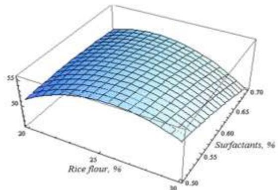
**Fig. 4. Response surface of dosing rice flour and surfactant on the porosity and viscosity of dough 800 Pa.s. for special purpose fondants**
